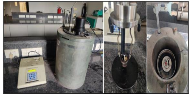
Figure 3: Assembly of Bomb Calorimeter
